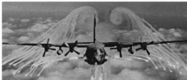
*Ejecting flares during a test of an infrared missile warning and self-protection system that was installed on a C-130 Hercules.*
